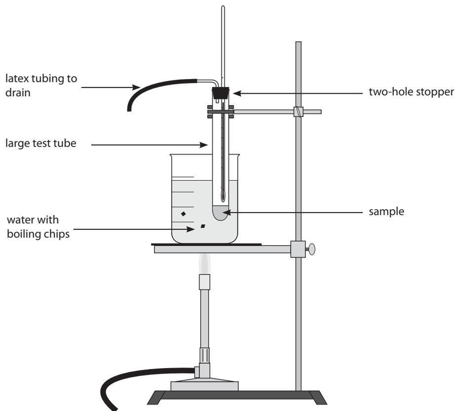
Figure 1-2. Boiling point apparatus.
