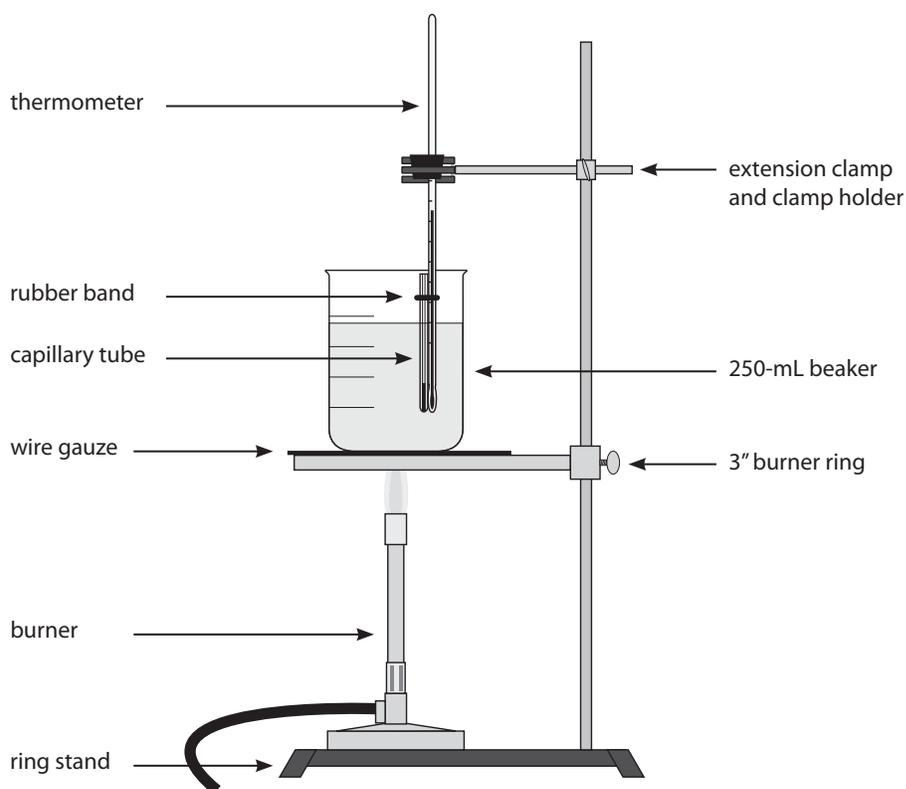
Figure 1-1. Melting point apparatus.
