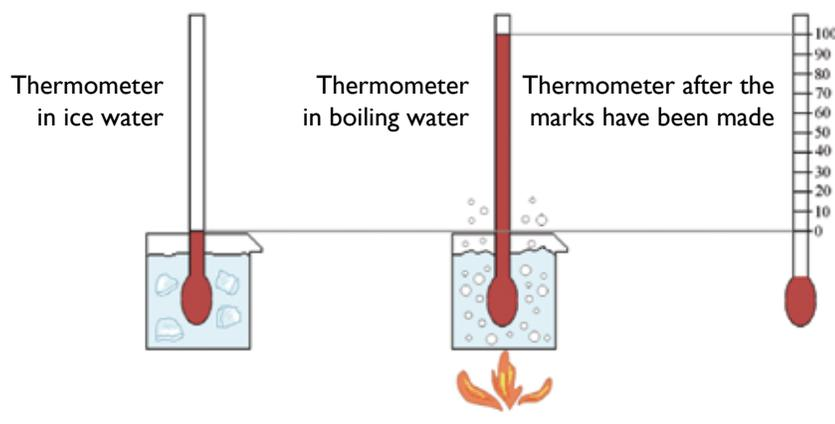
This process of using certain physical measurements to define the scale of a measuring device is called calibration. This particular calibration makes use of a surprising fact in chemistry:
