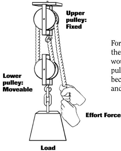
For example, with a system composed of 2 pulleys - one fixed and the other moveable – you need apply only **half** the effort force that would otherwise be needed to raise the load without the help of the pulleys, but you must pull **twice** the amount of rope. This is because the moveable pulley is supported by two sections of rope and you must move both sides of the rope to lift the load.
