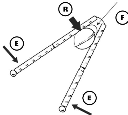
The nutcracker comprises two 2nd Class levers. The effort is applied by squeezing the two effort arms together by a hand; the load is the resistance of the nutshell to cracking; the fulcrum is the hinge.
