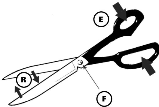
**A pair of scissors is an example of two 1st Class levers working together.**
