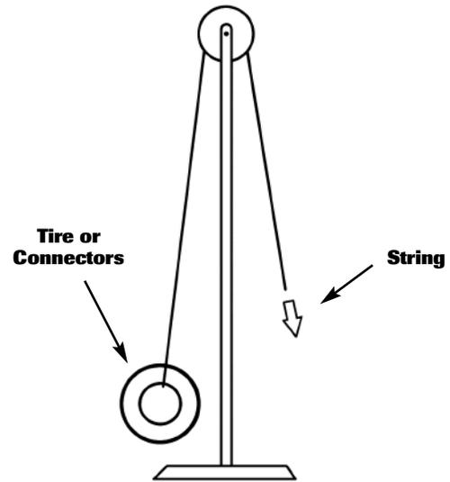
*Students should answer that when using the pulley, they pull down on the string to raise the load. It feels easier to pull down on the string using the pulley because "body weight" can also be used to help the pulling forces. When pulling upwards only "muscle" power can be used. In fact, the same amount of effort is used in both cases.*
