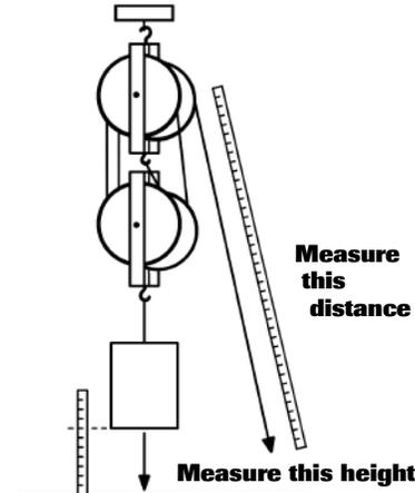
*Students should count 4 strings supporting the two movable pulleys. This means that this block and tackle makes it 4 times easier to lift the mass, but they also have to pull the rope 4 times further than if they were using a fixed pulley. Their results from Step 4 should have validated this: 10 pennies (the effort) could raise a load with a total weight of 40 pennies – the block and tackle made the job 4 times easier.*
