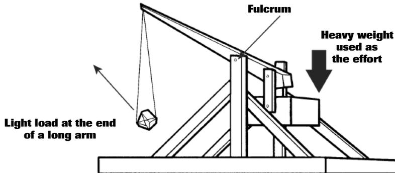
The trebuchet was a giant 1st Class lever in which the fulcrum was closer to the effort force. A massive effort force was pulled downwards several feet causing the long resistance arm of the trebuchet to move 20' or more at a high rate of speed. This motion propelled the small load a great distance at an even higher speed. Trebuchets caused enormous damage because they were able to toss boulders at castle walls at speeds in excess of 100 mph.
