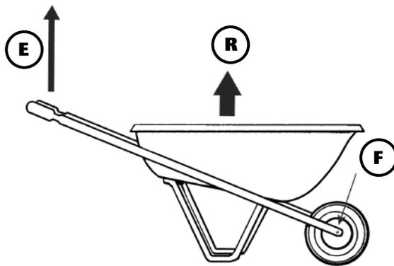
The wheelbarrow is a 2nd Class lever with the wheel acting as the fulcrum and the effort applied at the handles. The load is placed in the pan of the wheelbarrow, which lies between the effort and the fulcrum. (Fig 7.)
