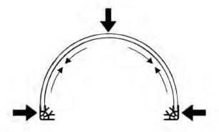
Fig. 30 - Reinforcing/strengthening an arch.
