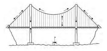
Fig. 50 - Forces acting on a suspension bridge.
