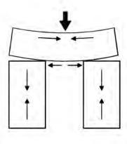
Fig. 33 -Forces acting on a beam bridge
