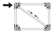
Fig. 25 - Compression acting on the strut.
