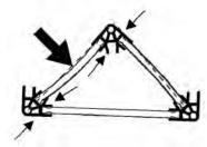
Fig. 26 - Force applied to the side of a triangle.
