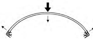
Fig. 29 - Force acting on an arch.
