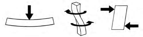
Fig. 9 - Bending: the combined effect of compression &tension
