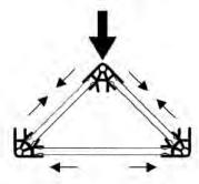
Fig. 27 - Force applied to the angle of a triangle.
