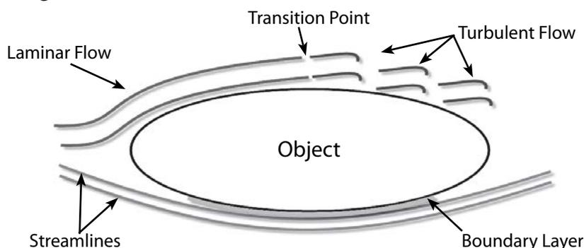
Drag is exactly what it sounds like. Drag slows down and is a hindrance in the flow of fluid.
