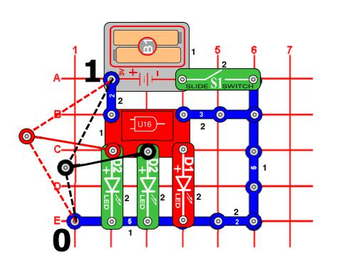
This circuit demonstrates how the AND Gate (U16) works. Connect one end of the red and black jumper wires to the A & B inputs on U16 and the loose ends to either low voltage (denoted as a "0") or high voltage (denoted as a "1"). If, and only if, both input A AND input B are high (both 1s, both gree LEDs on), then the Q output on U16 will be high (1), and the red LED (D1) will be on.
