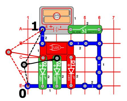
This circuit demonstrates how the Exclusive OR (XOR) Gate (U20) works. Connect one end of the red and black jumper wires to the A & B inputs on U20 and the loose ends to either low voltage (denoted as a "0") or high voltage (denoted as a "1"). If input A and input B are exclusive (i.e. different, one green LED is on and the other green LED is off), then the Y output on U20 will be high (1), and the red LED (D1) will be on.
