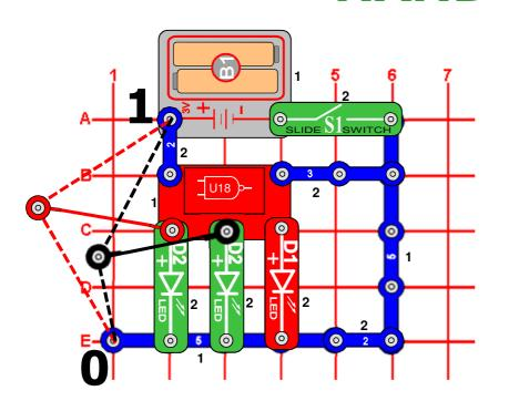
This circuit demonstrates how the NAND Gate (U18) works. Connect one end of the red and black jumper wires to the A & B inputs on U18 and the loose ends to either low voltage (denoted as a "0") or high voltage (denoted as a "1"). If either input A OR input B are low (0, either green LED is off), then the Q output on U18 will be high (1), and the red LED (D1) will be on. The output logic is exactly the opposite of the AND gate, hence this gate is called the NOT AND or NAND Gate
