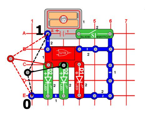
This circuit demonstrates how the NOR Gate (U19) works. Connect one end of the red and black jumper wires to the A & B inputs on U19 and the loose ends to either low voltage (denoted as a "0") or high voltage (denoted as a "1"). If, and only if, both input A AND input B are low (0, both green LEDs are off), then the Q output on U19 will be high (1), and the red LED (D1) will be on. The output logic is exactly the opposite of the OR gate, hence this gate is called the NOT OR or NOR Gate
