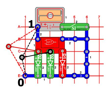
This circuit demonstrates how the OR Gate (U17) works. Connect one end of the red and black jumper wires to the A & B inputs on U17 and the loose ends to either low voltage (denoted as a "0") or high voltage (denoted as a "1"). If either input A OR input B are high (1, either green LED is on), then the Q output on U17 will be high (1), and the red LED (D1) will be on.
