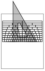
Using a triangle and T-square to line up the halves.
