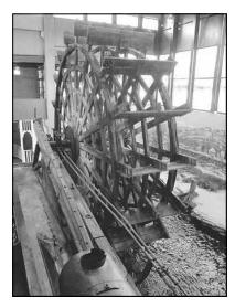
Side-wheel paddleboats and stern-wheel (wheel at the back of the boat) boats traveled America's big rivers. Some were oceangoing vessels as well. How did the boat move? Large paddlewheels churned the water and pushed the boat forward. What moved the paddle? Steamboats used steam to move rods, which were attached to the paddlewheel, much like rods pushed the wheels on a steam train.
