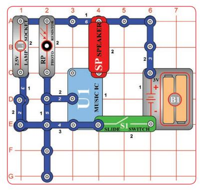
Build the circuit as shown. Place it where there will be no room light hitting the photoresistor (RP), such as under a piece of paper, or under the table. Turn on the switch.
