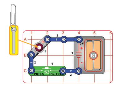
Build the circuit as shown, and place the iron core rod in the electromagnet (M3). Push the switch (S2) and touch the paper clip to the iron core rod in the electromagnet. Let go off the paper clip so only the magnet holds the paper clip in place. Release the switch (S2) to stop the flow of current.
