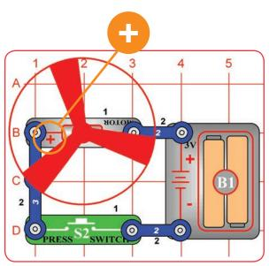
Note that the polarity of the motor is reversed. The positive terminal of the battery is connected to the negative terminal of the motor.
