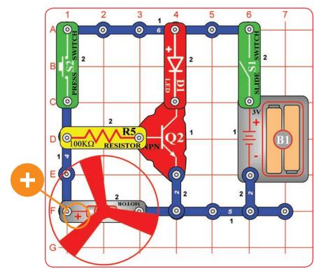
Build the circuit as shown. Place the motor (M1) with the "+" side to the left.
