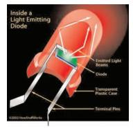
**LED - Light Emitting Diode**. A diode allows electricity to flow in only one direction, and only if the voltage exceeds a turn-on threshold. LEDs have a semiconductor inside, a material which only allows some electricity to flow. LEDs only need a small amount of electricity to light up so they are put in a circuit with a transistor. Many electronic devices use LEDs as indicator lights. They are often seen on CD players, televisions, and radios.
