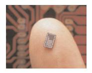
Integrated circuit - a circuit that has been made on a small semiconductor chip (silicon). It has many diodes, transistors and resistors which are very tiny. In this kit you have a blue music integrated circuit U1.
