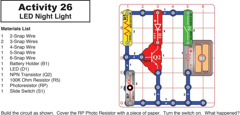
Remove the paper over RP and place the unit in the light. What happens? Place the circuit in a dark room. What happens? Turn on the room light. What Happens? \_\_\_\_\_ Is this circuit similar to an automatic night light? \_\_\_\_\_
