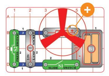
Build the circuit shown on the left. Place the motor (M1) with the "+" side as shown.
