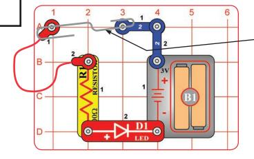
To make sure the circuit is working properly, place a paper clip across the opening between the two 2 snap wires as shown here. The LED should light up. When you place the paper clip across the terminals as shown, current flows from the batteries through the resistor, then the LED, then back to the batteries. The paper clip completes the circuit.
