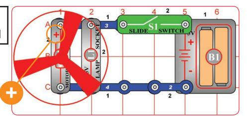
Build the circuit shown on the left. Place the motor (M1) with the "+" side as shown.
