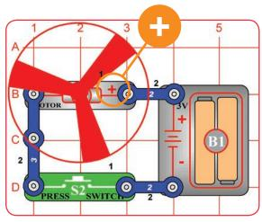
Build the circuit as shown. Place the motor (M1) with the "+" side on the right.
