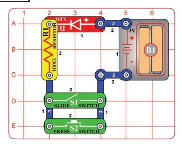
Use the table on the right to determine what happens for each combination. Enter under the heading "D1" the words "ON" or "OFF" for each switch Position shown on the left. This table is called a "Truth Table".
