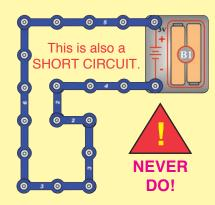
When the slide switch (S1) is turned on, this large circuit has a SHORT CIRCUIT path (as shown by the arrows). The short circuit prevents any other portions of the circuit from ever working.
