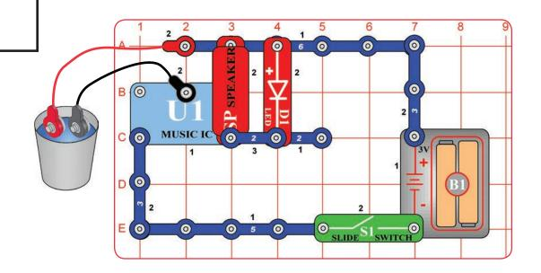
Build the circuit as shown, but leave the jumper wires out of the cup of water. Turn on the switch. What happens?
