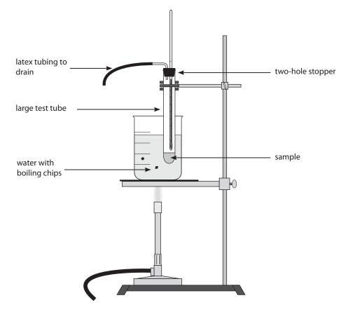
Figure 1-2. Boiling point apparatus.
