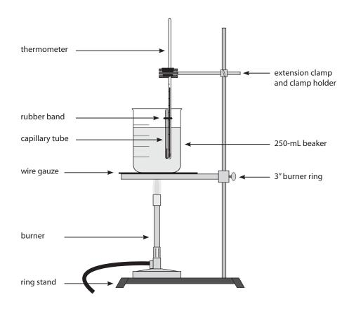
Figure 1-1. Melting point apparatus.
