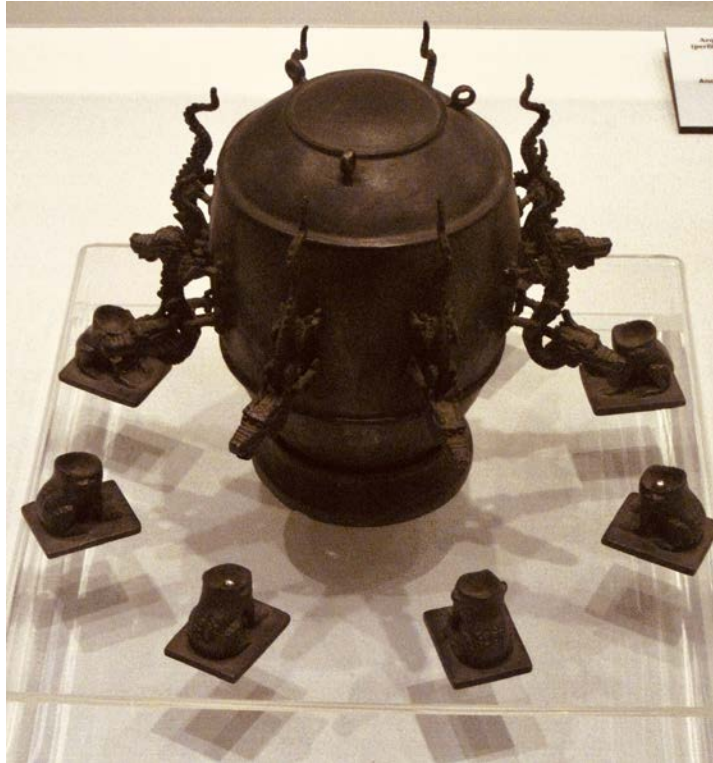
This replica Chinese seismograph shows four dragons facing north, south, east, and west. Sensing vibrations in the ground, the dragons were designed to drop a ball in the mouth of the nearest frog figurine—to indicate the direction of an earthquake!
