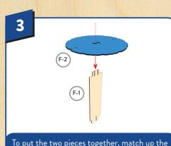
To put the two pieces together, match up the slots on each piece. Slide together.
