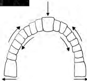
**Fig. 41 - Forces acting on an arch.**
