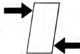
Fig. 11 - Shearing (sliding)
