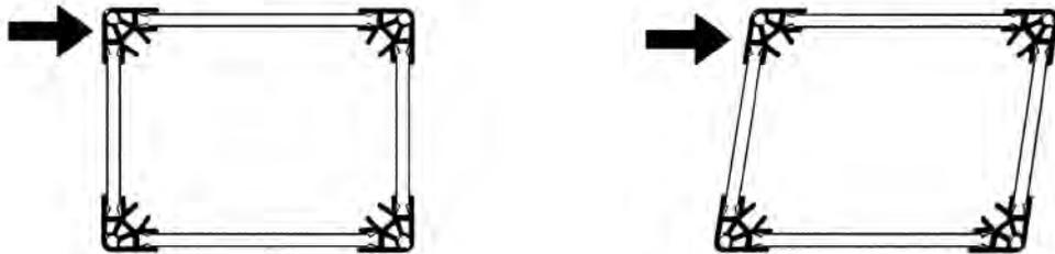
Fig. 23-24 - Rectangles: Pushing at a corner.
