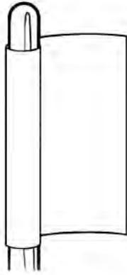
**Fig. 16i** - Roll the sheet of paper around a broom handle or large diameter dowling.
