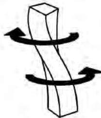
Fig. 10 - Torsion (twisting)
