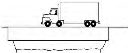
Fig. 4 - Strengthening beam by making it thicker.
