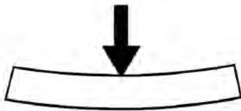
Fig. 9 - Bending: the combined effect of compression & tension
