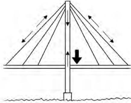
8. Refer back to previous work on strength and stability of bridge structures and talk about the possible problems engineers may have had to solve when designing and making cable-stayed bridges. For example, what might happen to the road deck as they build it outwards from the tower?
