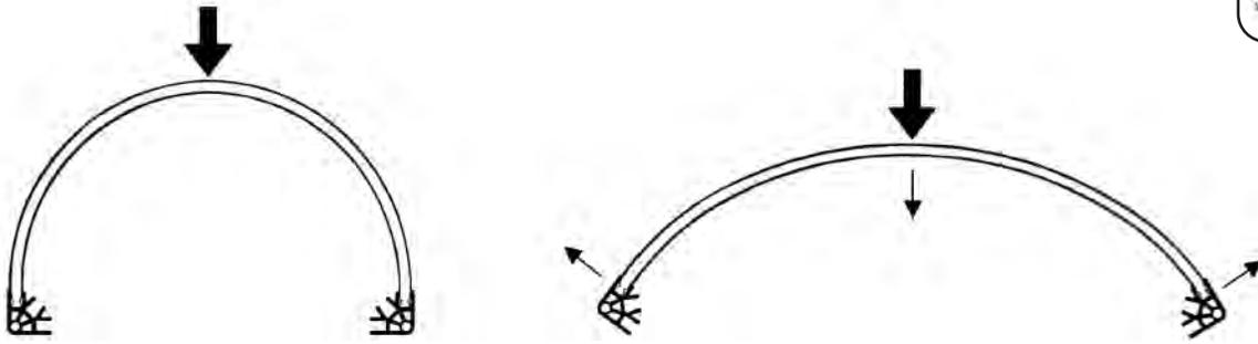
**Fig. 29 - Force acting on an arch.**
