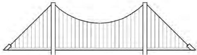
*Similarities: Both have decks suspended from cables. Both transfer load to the ground or bed rock using towers.*
