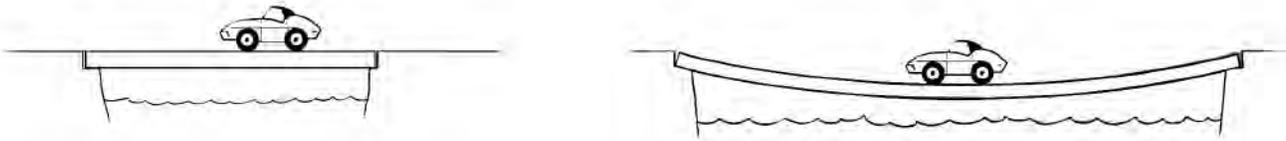
**Fig. 32 - Long beams are weaker than short ones.**
