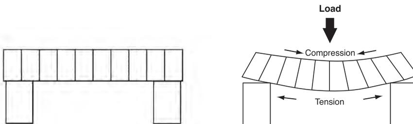
Fig. 12 - Forces acting on a beam.
