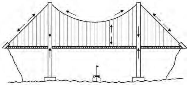
**Fig. 50 - Forces acting on a suspension bridge.**
