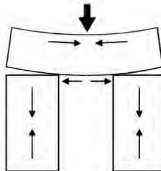
**Fig. 33 - Forces acting on a beam bridge.**
