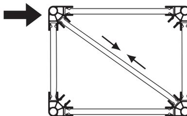
Fig. 25 - Compression acting on the strut.
