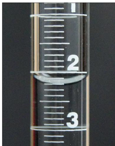
Figure 2.4. Reading the significant digits on a buret.
