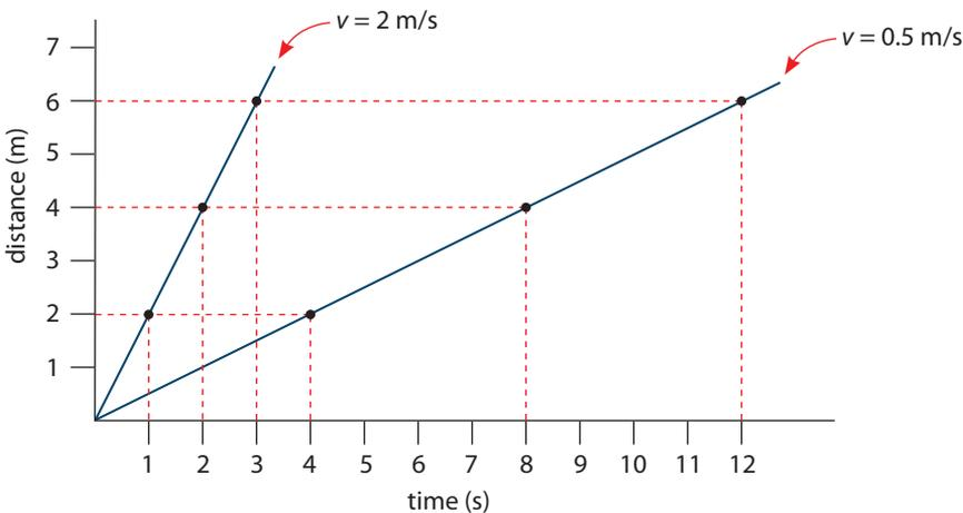
Figure 2.6. A plot of distance versus time for an object moving at constant velocity. Two different velocity cases are shown.
