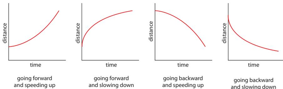
Figure 2.10. Curvature possibilities for distance vs. time graphs.
