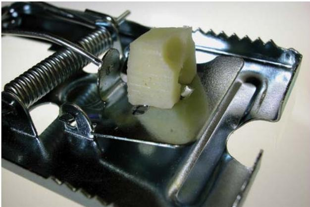
When a trap is set, the spring has potential energy.
