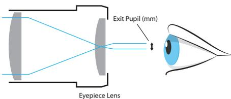
$$\text{Exit Pupil} = \frac{\text{Eyepiece Focal Length}}{\text{Telescope Focal Ratio}}$$
