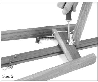
Locate Support Leg (G) with hinge. Align hinge with 2 pre-drilled holes on Top Cross Bar (C). The hook that is attached should face the mast as you attach with 2 of the Short Screws (N).
