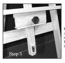
Step 5: Add Tray Stop (O) by securing with 2 Round-Headed Screws (P) to the bottom of the mast.
