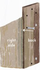
5. Attach roof to front, and then to back. There will be a  $\frac{1}{4}$  gap between roof and top of sides to allow for airflow.
