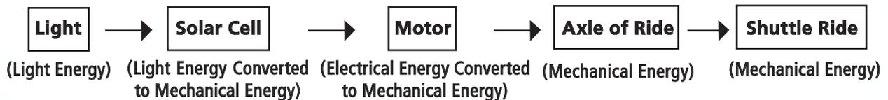
**(The light produces light energy – solar cell (converts light energy to electrical energy) – electricity travels through the wire to the motor – the motor converts electrical energy to a form of mechanical kinetic energy.)**
