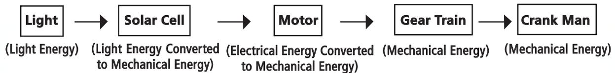
(The light source produces light energy— the solar cell [converts light to electricity] – the motor converts electrical energy to mechanical energy – the Crank Man moves in response to the mechanical energy provided by the gear train.)
