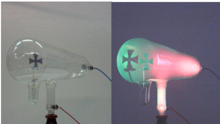
Crookes tube without the electricity turned on.
