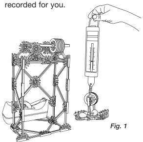
Multiply the force of the weighted tray by the distance that the tray moved. Record your calculation in Table 1. This is the amount of **work** done by the machine (work output).
