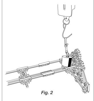
5. Based on your calculation for mechanical advantage, **predict** the amount of force that you must exert to pull the mass up the ramp. Write your prediction on the worksheet.
