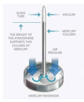
How a Mercury Barometer Works
