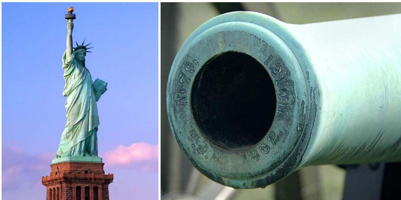
The Statue of Liberty (left) turned bluish-green because hydrogen, oxygen, and carbon atoms from various substances in the air have combined with copper atoms to make copper hydroxycarbonate. This Civil War cannon (right) is made of bronze, which is a mixture of copper and tin. The copper in the mixture has also reacted to form copper hydroxycarbonate.
